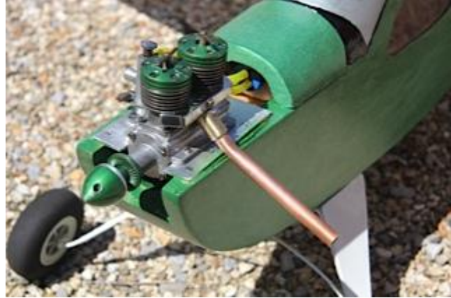
Exhaust extension, a previous owner had sawed the original off leaving a very small stub
