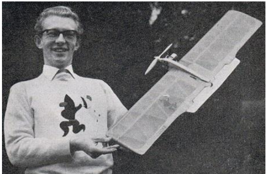
The designer's model, with Kenton club emblem displayed in due prominence. Note the slotted elevator on this earlier model is of greater span.
