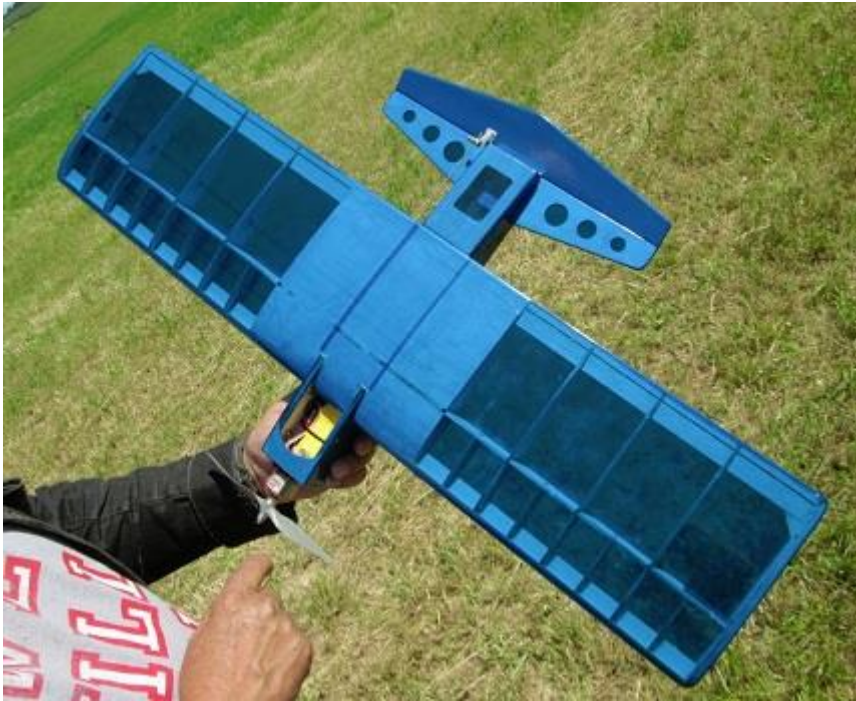
Underside view of the model showing easy access to ESC, and ventilation
