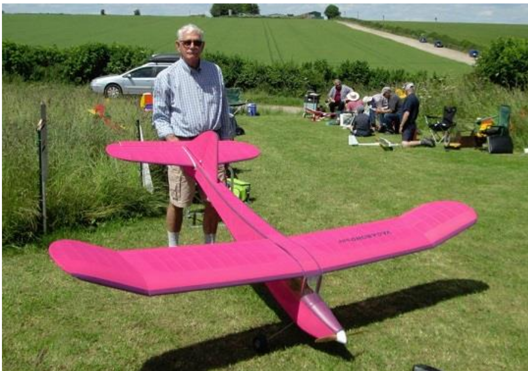
John Laird with his new enlarged Vagabond giving scale to this Chiffon covered electric model
