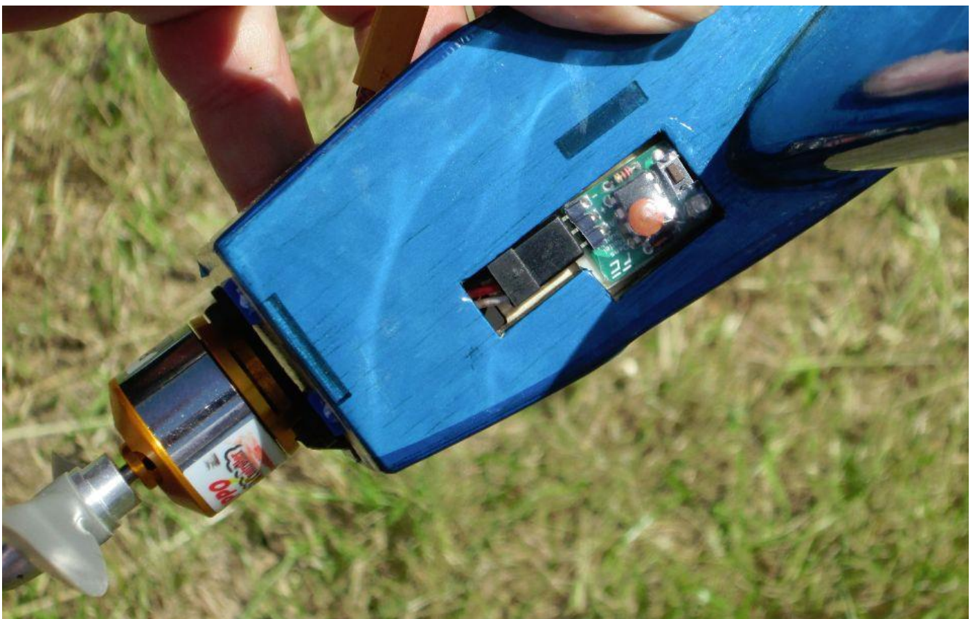
Den's Dynamo showing the Eze timer he also sells. He limits the flight time at present to 3 minutes and that is a long enough for a fast perky model unless you are a hardened combat flier.
