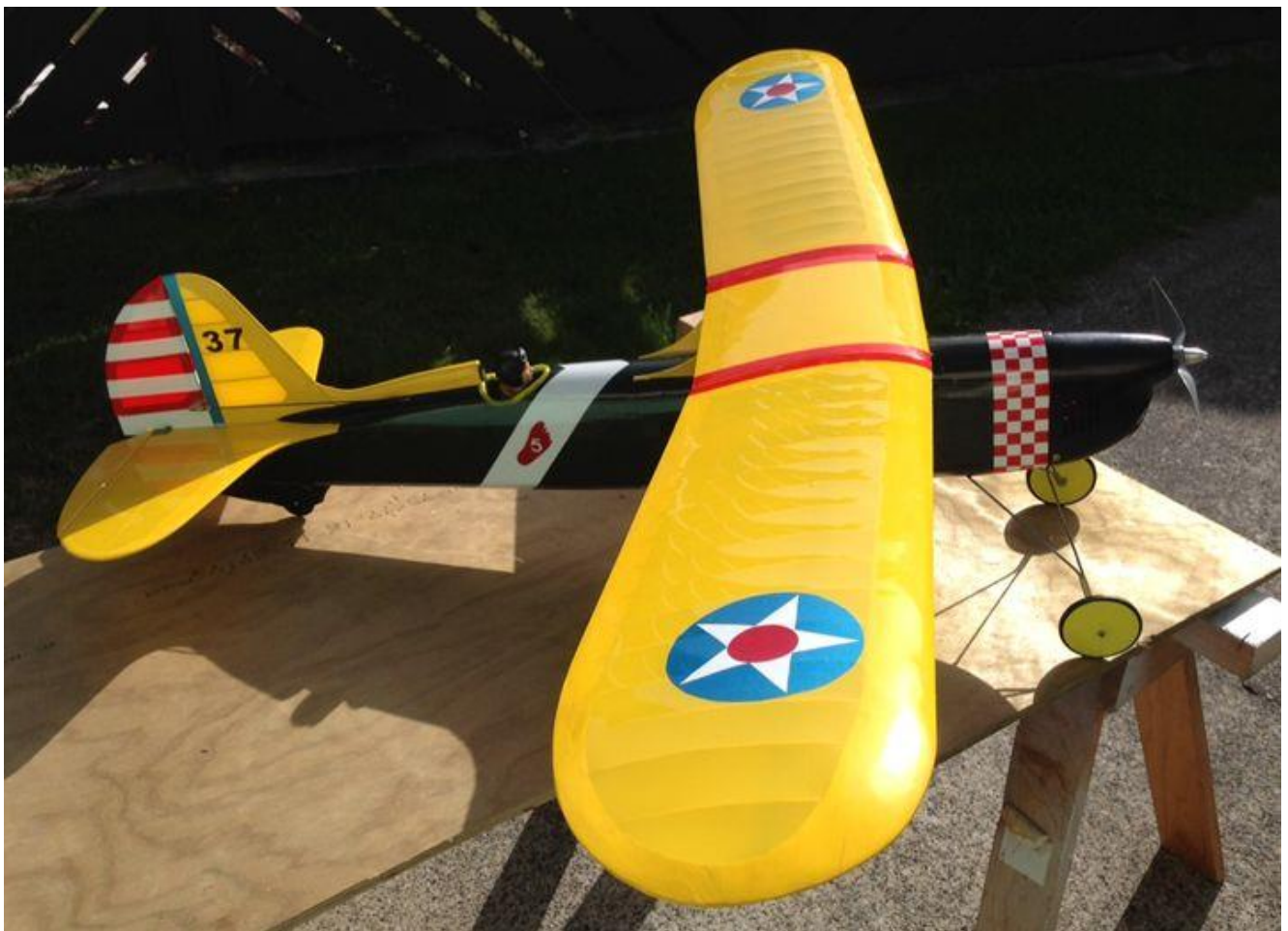
My 5 Foot Gas model uses hand-cut film too. Those roundels are made up of 3 layers to get the multi colours. The chequered cowl wrap is a strip of sticky decal though.
