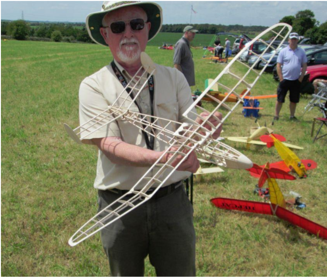
Richard Farrer with his current project for RC all controls for this Invader glider are via the main wing as you can see, for turning, the wings pivot thus acting as ailerons whereas elevator is taken over by increasing / decreasing the angle, decalage, of the main wing.
